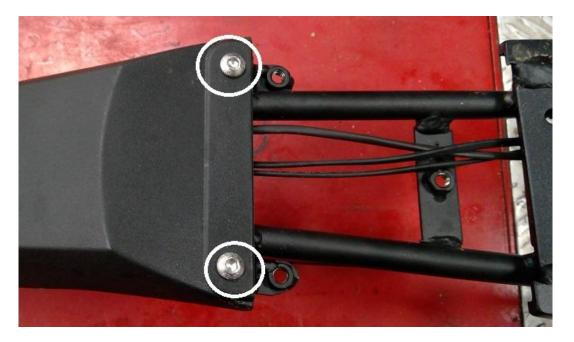
9. Separate the subframe halves by removing the 2 nuts and bolts (M6  $\times$  16mm, self locking nuts) and separate the components.
