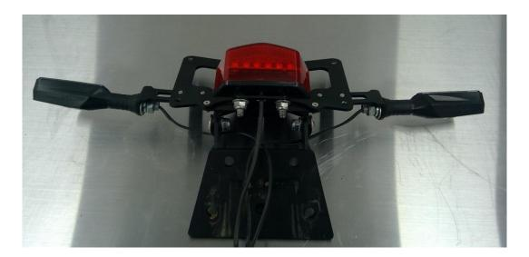
Ensure the lighting wiring is fitted inside the modified subframe as shown before refitting the saddle underside cowling.
